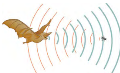
Figure 14.8 A bat uses sound echoes to find its way about and to catch prey. The time for the echo to return is directly proportional to the distance.
